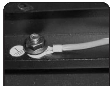
**7** Attach other end of the #10 wire to the bonding post located at the middle of the lower horizontal support using the M6 flange nut provided.
