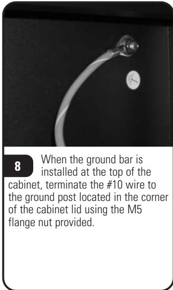
**8** When the ground bar is installed at the top of the cabinet, terminate the #10 wire to the ground post located in the corner of the cabinet lid using the M5 flange nut provided.
