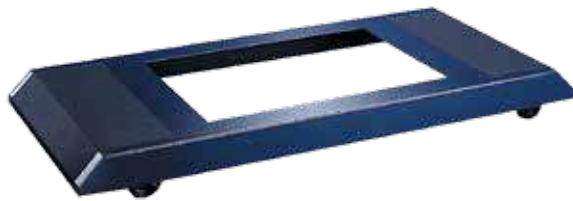
Mobile Bases fit 600- and 800-mm wide frames. They extend beyond the front and rear of 600-mm cabinets to provide enhanced stability. Provides front extension only on 800-mm cabinets. Constructed of steel finished in RAL 9005 textured black polyester powder paint. The base fastens to the underside of the frame and provides integral mounting of furnished casters. The front and rear top surfaces of the base are trimmed with black rubber mats 3-mm thick.
