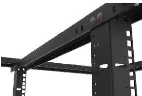
Rack angles are sold in pairs that are RU marked on all sides. One side is tapped 10-32 while the other side is square hole (.375 x .375 in.). Both sides are spaced per EIA universal standard. Rack angles may be assembled in either tapped or square-hole configuration. Rack angles and mounting brackets are formed from heavy gauge steel and are polyester powder painted low-gloss, RAL 9005 black. All hardware and brackets are included for assembly into cabinet.
