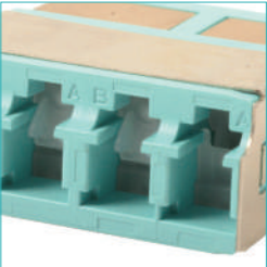
Shuttered LC Adapters Small plastic shutter door that opens upon insertion, without touching the connector end face, and springs back into the closed position upon removal to ensuring protection of empty ports.
