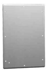
Constructed of 12 gauge steel and designed for use with 10 gauge and 12 gauge enclosures. Provides a removable cable egress and entry plate while maintaining UL/NEMA integrity of the enclosure. Gasket with pressure-sensitive adhesive is included to be applied after desired modifications are completed. Finish is ANSI 61 gray polyester powder paint. Maintains UL/NEMA Type 4 and Type 12 if properly installed in an nVent HOFFMAN enclosure.
