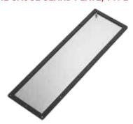
Mild steel gland plates are constructed of 12 gauge steel and finished with ANSI 61 gray polyester powder paint. Gland plates provide a removable cable egress and entry plate while maintaining enclosure rating of UL Type 4 and Type 12. Easy installation by cutting a rectangular opening in the enclosure and fastening with included hardware kit.
