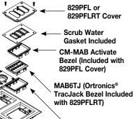
MAB3S2 Bezel (Ortronics® Series II Bezel Included with 829PFLRT) Fiber Optic Installation (Activate Only).
